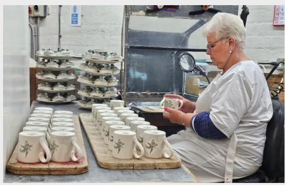
Transferring the Burleigh mark on mugs.
